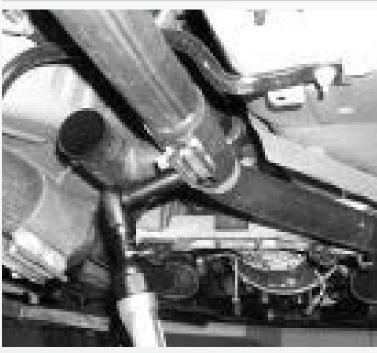
Separate the cat-back system by loosening the 2 nuts on each band clamp and prying the locking tabs up with a small screwdriver while sliding the clamp towards the rear of the car.
