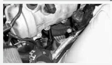
Remove the stock exhaust manifold and gasket. (Some of the manifold bolts are easier to access while working under the hood)
